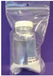
Sterile, clear plastic sample bottle containing Sodium Thiosulfate Powder inside Zip seal bag with absorbent
